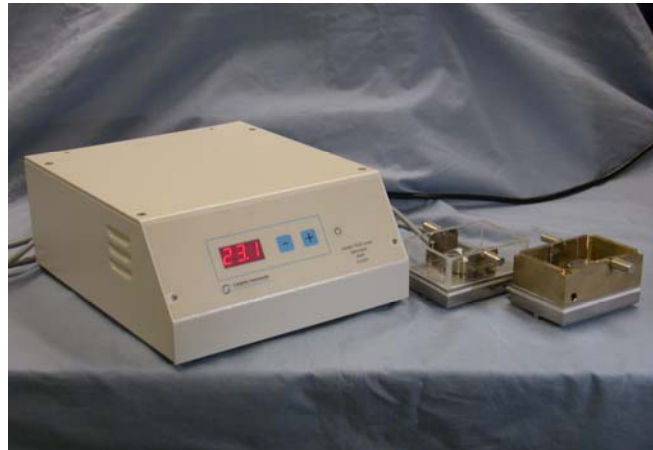
7600 controller with alternative standard and sterilisable cooled tissue baths
