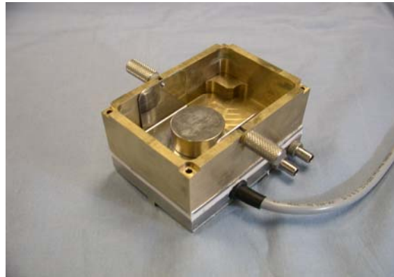
7600S Tissue bath with removable, autoclavable piece,
