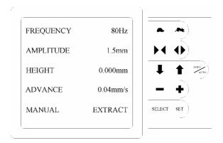
Figure 8 Manual mode display
