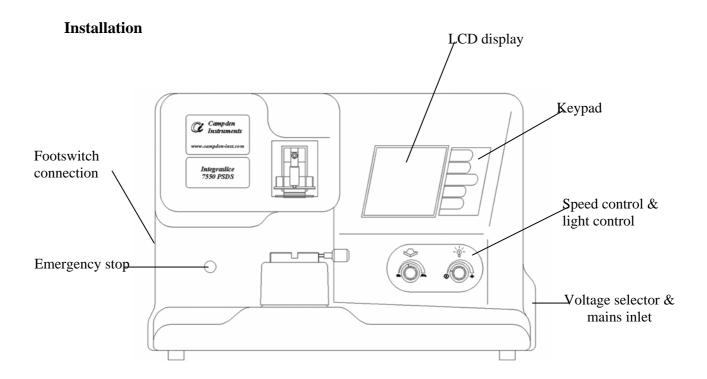
Figure 1 Front view of the Integraslice
