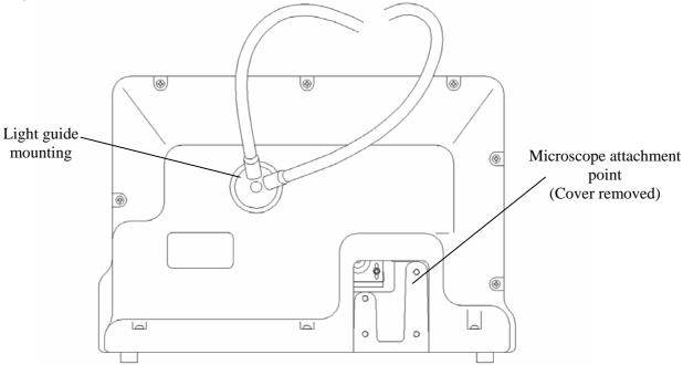
Figure 2 Rear view of the Integraslice
