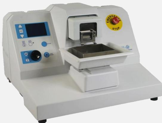
Our top of the range high precision, vibrating microtome (vibratome for short), this is the finest tissue slicer in the world for preparations for visual patch clamping or high-resolution imaging.
