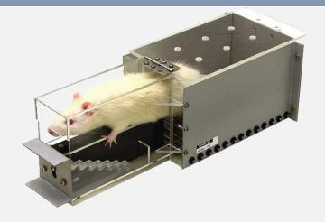
This staircase apparatus provides a simple, efficient, and easy way to quantify the testing of skilled paw reaching for the rat.
