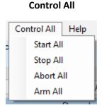
The Control All menu provides controls for starting, stopping, and aborting all channels.
