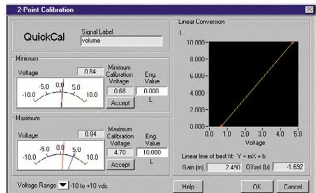
5. Set the bellows so that the scale reads 0 liters. Click the Accept button for the Minimum Calibration voltage.
