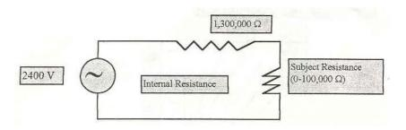
When the subject's resistance equals 100,000 ohms the current flow is 1 mA. When the subject's resistance equals 0 ohms the current flow is 1.04 mA. In this case the % regulation is 4%, well within reasonable specifications. The higher internal resistor clearly gives better regulation; however, the transformer voltage must be boosted slightly to compensate for the higher resistance. 2500 volts has been found to be an optimum value and is thus incorporated in the Lafayette shocker.
