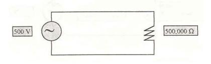
The current flow through the resistor would be given by I = E/R or I = 5,000/500,000 = 1/1,000 Ampere or 1 Milliampere (mA)
