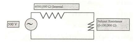
The current is equal to 500/500,000 (400,000 + 100,000) or 1 mA when the animal is unexcited; however, when the subject's resistance drops to 0 ohms, the current is equal to 500/400,000 or 1.2 mA.
