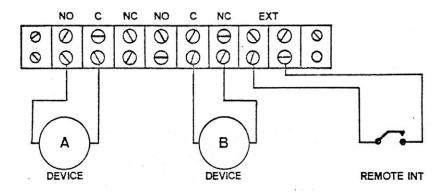
6. Initiate the time interval either by momentarily depressing the front panel push-button or the remote initiate switch.
